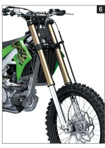
\* Kashima Coat creates a hard, low-friction surface on the fork outer tubes. The hard coating helps prevent wear abrasion on the inside of the tubes, ensuring the sliding surfaces remain smooth for a long time, while the outside is protected against corrosion. The lubricating material in the coat contributes to smoother suspension action (especially at the initial part of the stroke) and a better ride feel.
