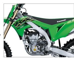
\* Slim aluminium perimeter frame is a lightweight construction composed of forged, extruded and cast parts.
