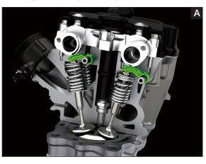
\* Complementing the aggressive cams, large-diameter intake (ø32 mm) and exhaust valves (ø26.5 mm) with high lift (IN: 10.3 mm; EX: 9.1 mm) flow a high volume of air, contributing to high-rpm power.
